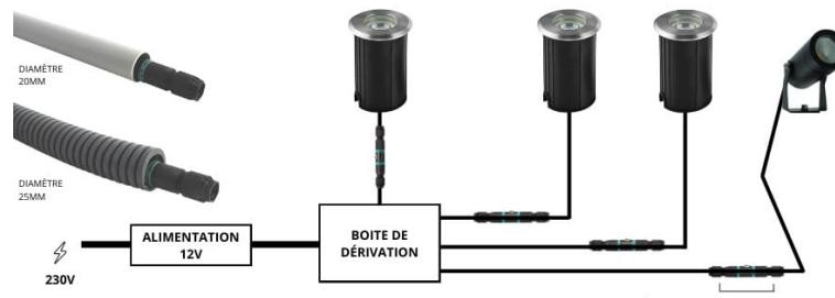
MINI CONNECTEUR ÉTANCHE DE JONCTION RAPIDE IP68 - TECHNO THB.381 DANS GAINÉE DE 25 MM
